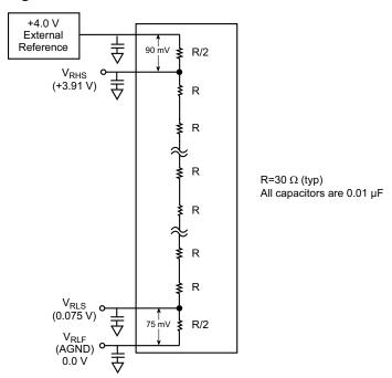
force and sense lines to AGND with a .01  $\mu$ F capacitor (chip cap preferred) to minimize high-frequency noise injection. If this simplified configuration is used, the following considerations should be taken into account.
